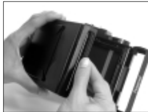
E) Check the film exhaust outlet and remove any contaminants such as paper or dried developer.
