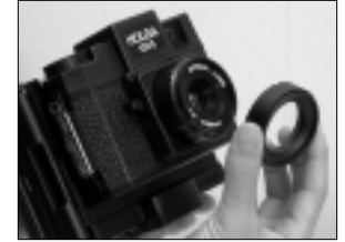
Always cover the lens of the camera with the attached correcting lens.
