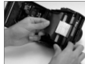
Check the number of pull tabs located under the lightproof paper. The number of pull tabs equals the number of pictures.
