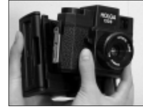
Replace the back cover of the camera with the Polaroid holder.
