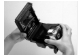
Load the new film with the lightproof paper facing forward.
