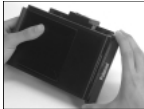
F) Close the Polaroid holder cover.
