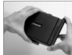
Hold the upper and lower ends of the Polaroid holder latch and rotate outward.
