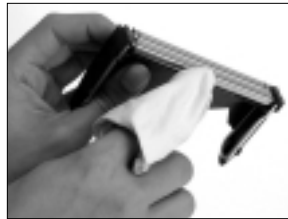
C) Clean the detached roller using non-fray cloth.
