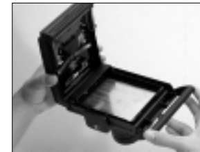
Open the Polaroid holder cover.
