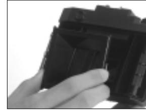
Replace the frame already fixed to the camera with the 6x6 frame included with the holder. Fix to inside of camera.
