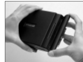
Ensure that the lightproof paper is protruding out of the holder before closing the cover.
