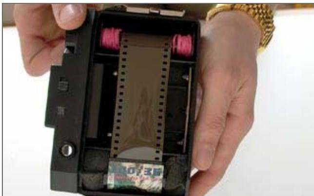
Smash your 35mm film cartridge into the middle of this. The fit should be tight - your film cartridge must not be able to move up or down. Ensure that your left-side to right-side alignment is good, and that your film transports straight across.
