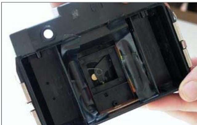
Opening the back of your Holga, insert two "AA" batteries to power the flash. As the strange Gods of Design would have it, the Holga batteries are not held in place by any kind of spring or tension. This is just the first of many useful applications for your opaque tape - go right ahead and securely tape those batteries inside; or they will roll around inside the camera. Be sure that your tape doesn't obscure the square surrounding the shutter hole.
