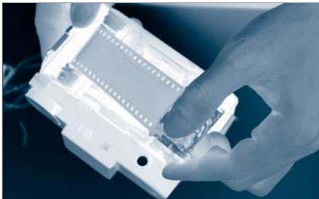
Remove the tape and open the Holga's back. Again, there must be no light around at all. Pick up your film spool with two fingers. GENTLY tug the film upwards, grasping only the cartridge body, and pull the bottom of the take-up spool out of its cradle.
