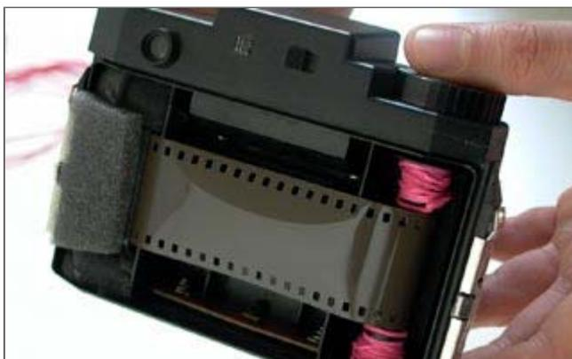
Using a small piece of tape, secure the flat strip of foam to the top of your film cartridge. This prevents the cartridge from moving out of its soft little housing.
