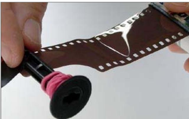
Place your film leader in the middle of your now-rubber-banded-take-up spool. Use a small piece of tape to secure it in place. Wrap the film around the take-up spool 3 or 4 times, making sure that it is T-I-G-H-T! Place the take-up spool into its right-side compartment.
