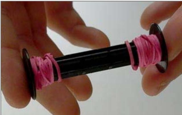
Remove your take-up spool on the left side. Wrap a few thin rubber bands around the top and bottom, leaving no less than 3.5cm (1.35in) in the middle. Your 35mm film leader will fit snugly in this space, with the rubberbands preventing it from moving up or down
